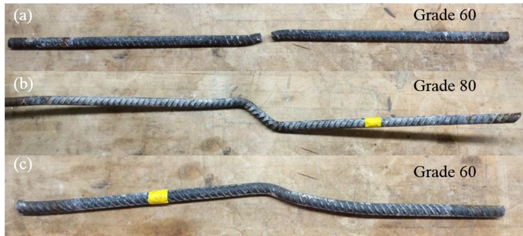
FIGURE 22 – Steel Failure and Deformation: (a) 135°; (b) 45°; (c) 90°
